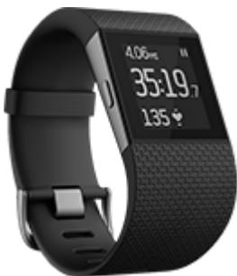
**The device that I have chosen is the FitBit Surge**, which tracks, steps taken, heart rate, miles walked, calories burnt, and floors walked up. It also keeps track of how well I sleep, noting times that I awoke during the night and also when I was restless. It tracks sleep efficiency as well as many other functions. It is more powerful than anyone would need for the NEAT program, however, if your plan is to move on up to an exercise program, in the future you may want to consider it.
